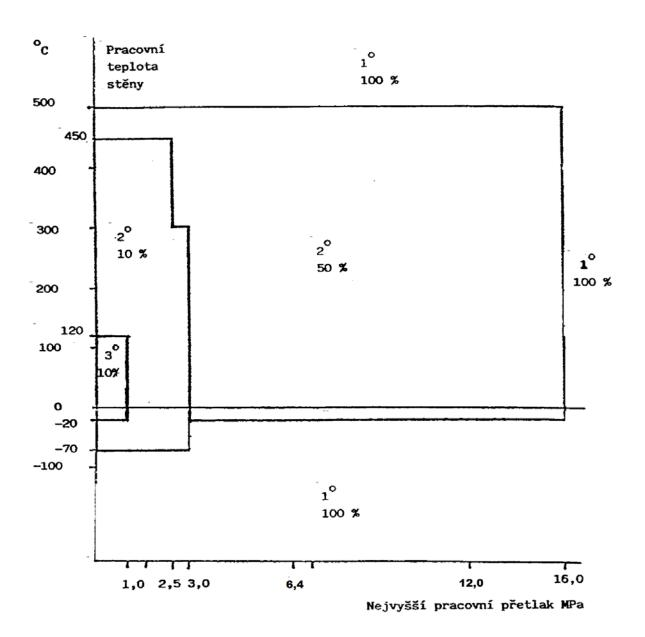
Picture No. 2 -Acceptable weld classification levels and test extents of pipelines with hazardous operation media if people are endangered and if there is an increased risk environment in relation to operation pressures and temperatures.
