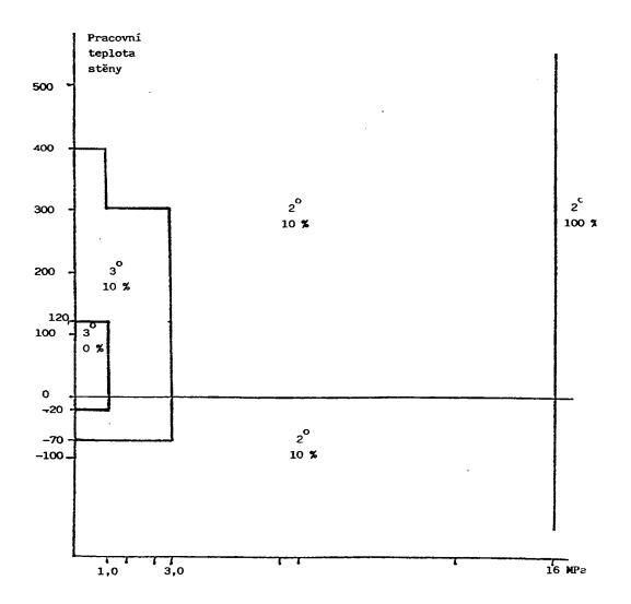
Picture No. 4 -Acceptable weld classification levels and test extents in relation to operation pressure - temperature for pipelines with other operation media.
